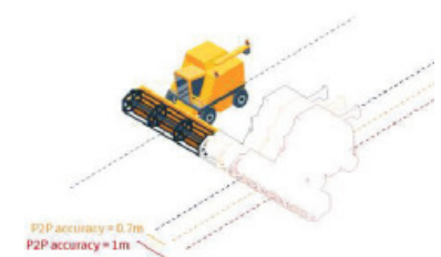
PASS-TO-PASS (P2P) accuracy concept.
