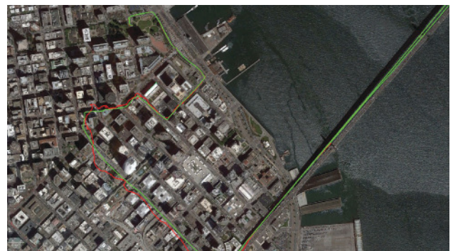
FIGURE 2 The result of supercorrelation on positioning performance in the urban canyons of central San Francisco. The red line is a standard state-of-the-art vector tracking GPS solution, and the green line is the same positioning engine with supercorrelation processing enabled.
