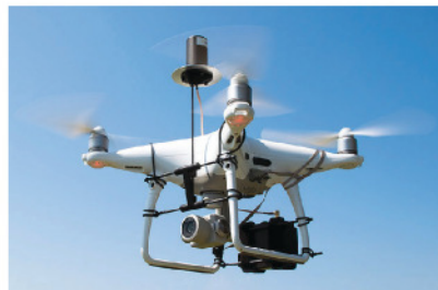
DJI PHANTOM 4 Pro with Loki PPK system.
